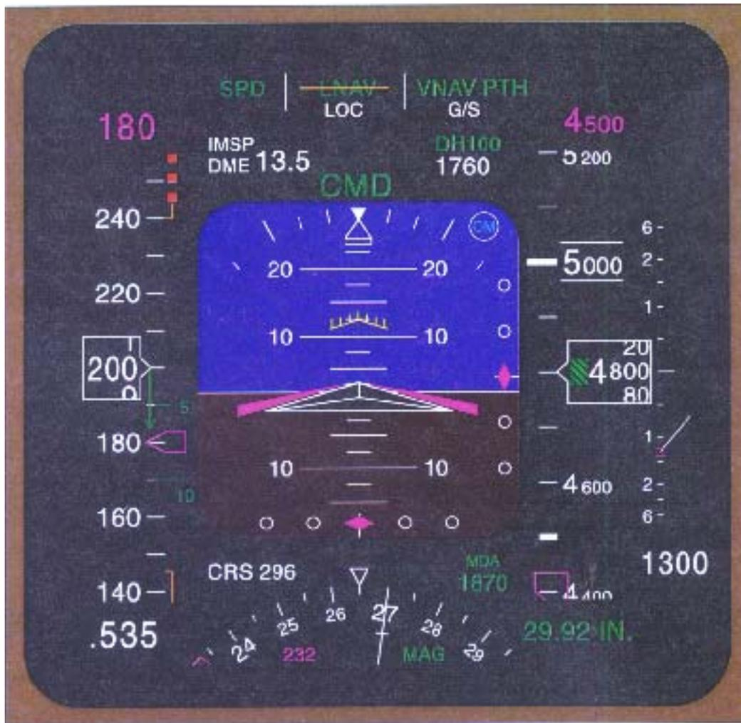
Ironically, as Hutchins shows, they do not reflect perceptually at human scale the differences in speed and positioning of slats and flaps, even though formally they contain all the information. For the old gauge, the gross physical configuration of the display was different for different speeds, and different entire regions of the display corresponded to the different positioning ranges, but in the new display, the gross physical configuration of the display does not change.
